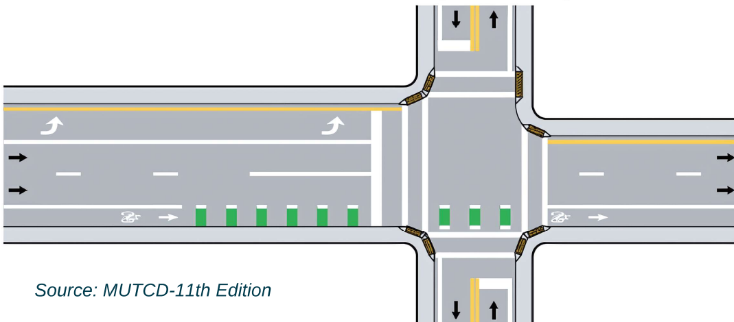
D – Applied supplementing the dotted line approaching intersections and/or the dotted extensions of bicycle lanes through intersections
