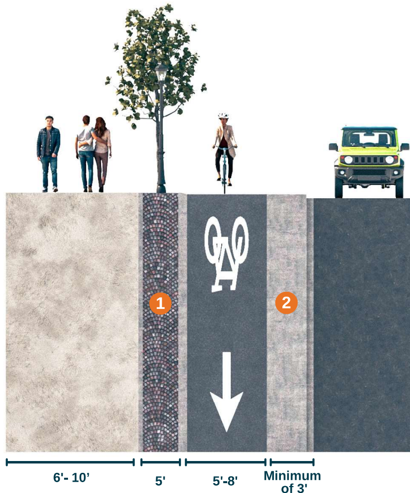
One-Way Separated Bike Lane with Poured Median
